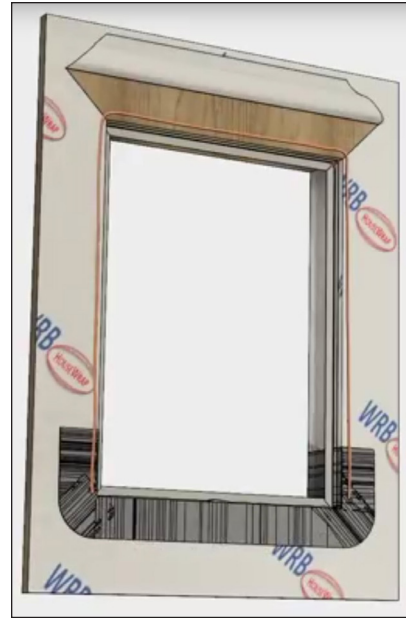
8. The rough opening is now prepared to set the window
